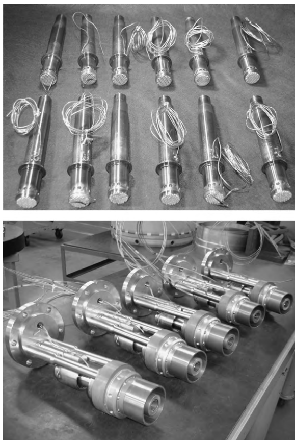
Fig. 4. Catalytic pilot hardware. (a) Set of 12 instrumented catalytic pilot cartridge assemblies. (b) Catalytic pilots integrated with T70 swirler assemblies.
